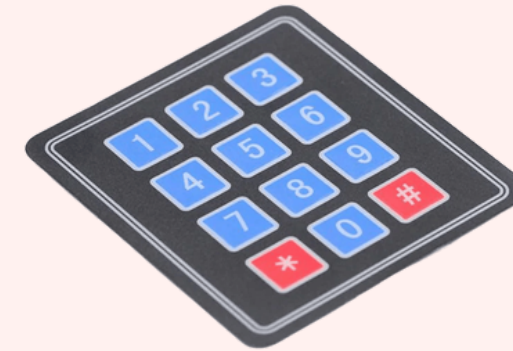
3*4 keypad module - For opening the door.
