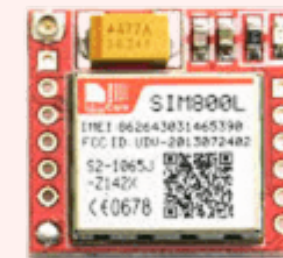
GPRS GSM SIM800L module - Wireless communication
